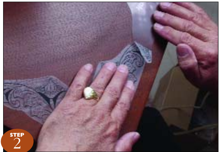
STEP 2 Peel and cut off part of the backing on the stencil before applying the rest of the stencil to the tabletop. Work any air bubbles out as the rest of the pattern is applied and rubbed onto the tabletop. Examine the pattern closely. Depending on the quality of the photocopied pattern, use a pencil to add a few lines.
