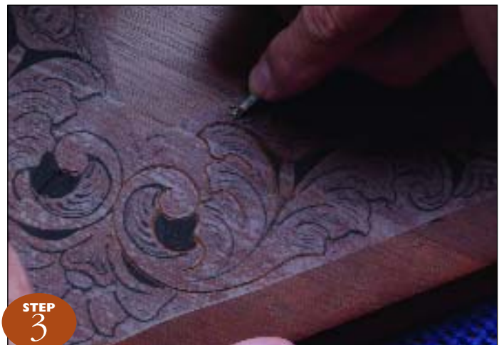
STEP 3 Using a \frac{1}{8} " 60-degree V tool, begin carving on the right side of the pattern, toward the middle, at a depth of \frac{1}{32} ". Use this tool for all of the initial outlining of the pattern.
