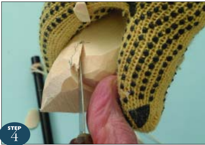
STEP 4 Start to define the face by removing wood with a press cut as shown in the photo.
