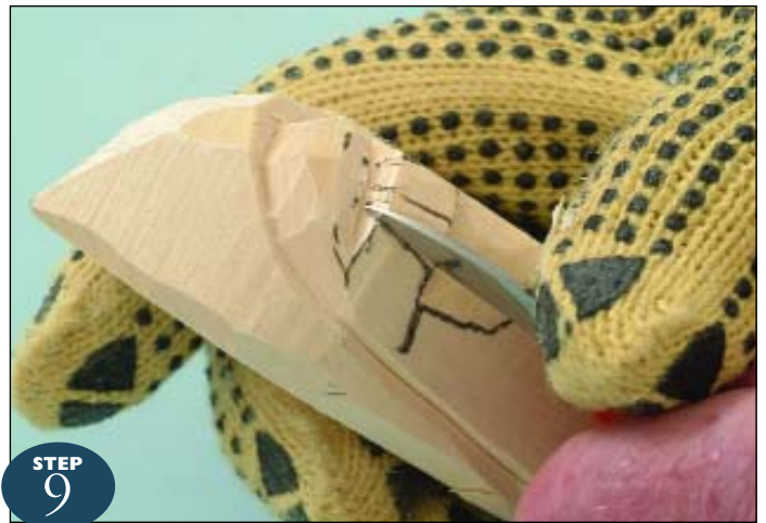
STEP 9 Set the knife into the wood straight in so you see only the back of the blade and follow the 8 o'clock line. Lay the knife onto the flat plane and clean out the cut.
